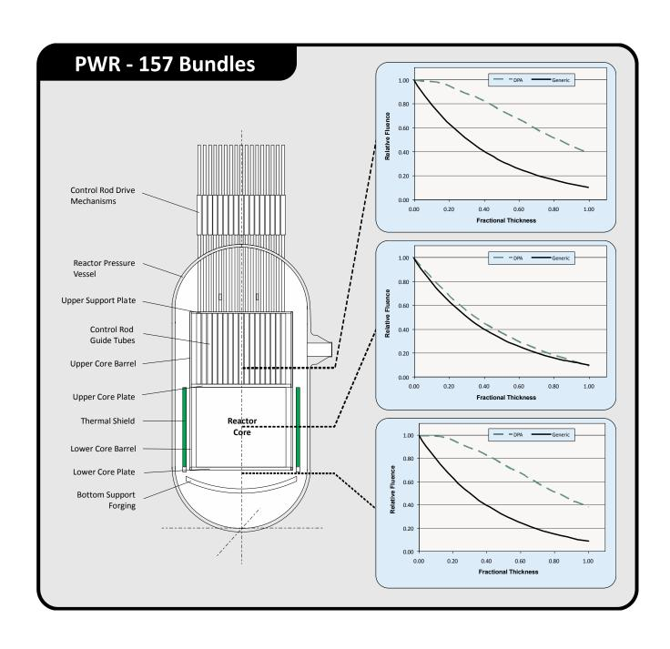
Fig. 4 – PWR with 157 Fuel Assemblies
