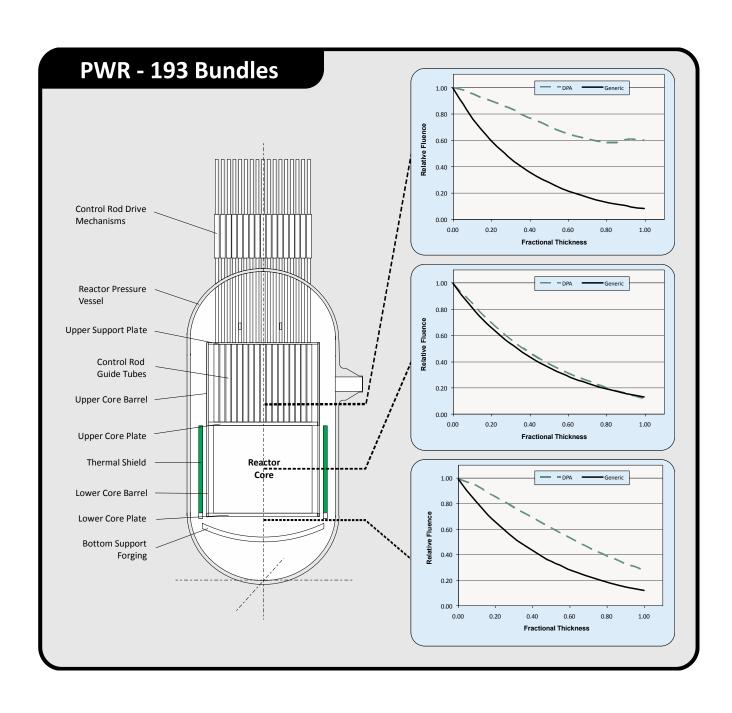
Fig. 5 – PWR with 193 Fuel Assemblies
